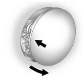
The cap is behind a locking fuel door on the passenger side of the vehicle. The fuel door is locked or unlocked every time the driver's door is locked or unlocked with the power door locks or the transmitter.
